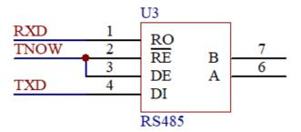
In the figure, TNOW is the switch pin, the TNOW pin can be used to control DE (active high and transmit enabled) and RE# (active low and receive enabled) pin of RS485 transceiver. RS485 transceiver should use the same power supply as VIO.
